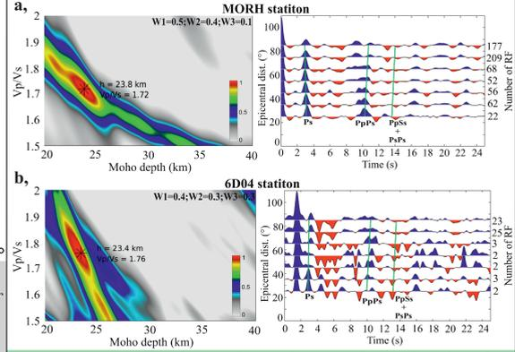
Figure 5. H-K grid search results a, MORH (hard rock); b, 6D04 (sedimentary) station.
