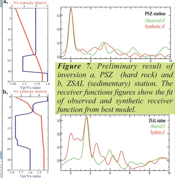
Figure 7. Preliminary result of inversion a, PSZ (hard rock) and b, ZSAL (sedimentary) station. The receiver functions figures show the fit of observed and synthetic receiver function from best model.
