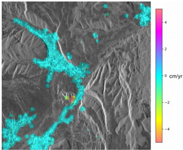
First results show deformation on the southern flanks of the salt diapir. Subsidence is in the 3 – 4 cm/yr range. Lack of scatterers on the top of the salt diapir → artificial reflectors.
