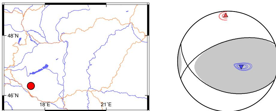
*Left:* Epicenter location. *Right:* Beach ball representation of the obtained source mechanism. Compressional quadrants of the optimal solution are shaded. Contours represent the 50, 68, 90 and 95% confidence zones for the P (red triangle) and T (blue inverse triangle) principal axes. Equal area projection of lower hemisphere is used.
