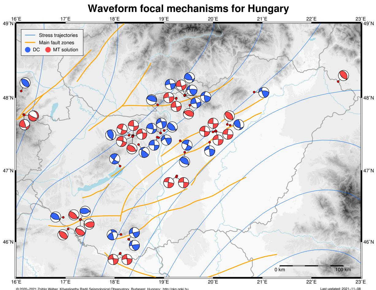
Figure 1: Source mechanisms of the analyzed earthquakes on a map of Hungary (red: MCMT solutions; blue: JOWAPO solutions; shaded area: compression; open area: dilatation). Equal area projection of lower hemisphere is used. Thin blue lines depict the trajectories of maximum horizontal stress directions after Bada et al. (2007), whereas thick orange lines indicate main active fault zones after Horváth et al. (2006).
