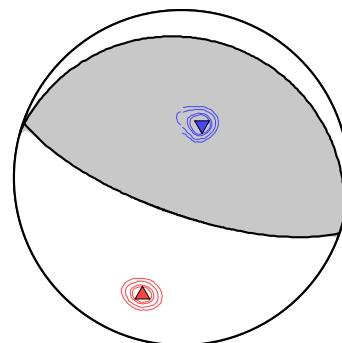
*Left:* Epicenter location. *Right:* Beach ball representation of the obtained source mechanism. Compressional quadrants of the optimal solution are shaded. Contours represent the 50, 68, 90 and 95% confidence zones for the P (red triangle) and T (blue inverse triangle) principal axes. Equal area projection of lower hemisphere is used.
